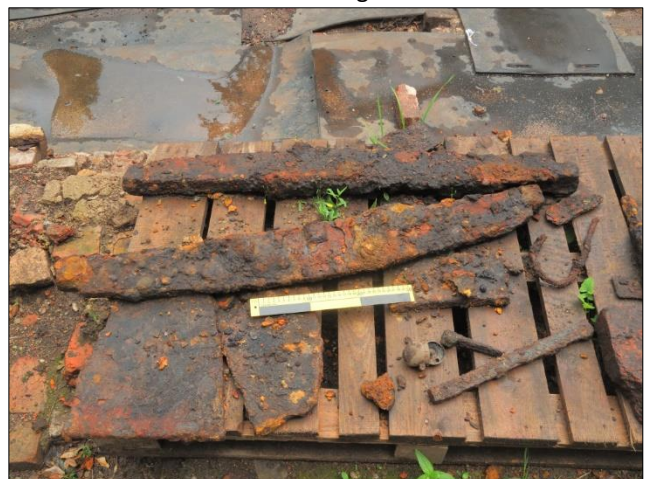
Photo 27 – Two complete firebars were found when removing spoil from the most north-easterly part of the New Boiler excavations. (30 cm yellow/black scale)
