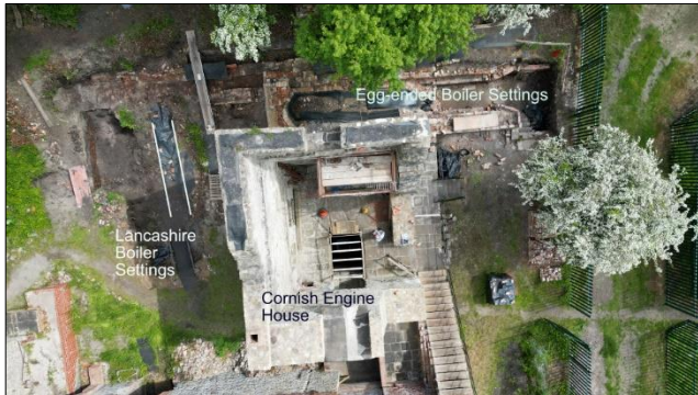
Photo 10 – Annotated aerial photo of the Cornish Engine House (middle), Egg-ended Boiler settings (top right) and Lancashire Boiler settings (left), taken in May 2023. (Drone photo © Toby Hore, 2023)
