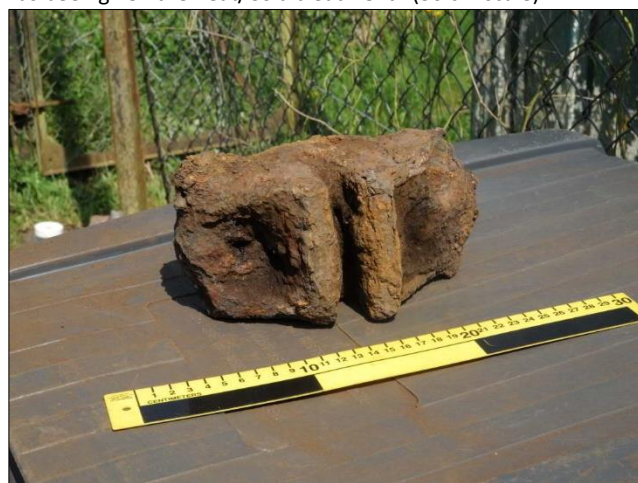
Photo 14 – A light gauge railway chair found in the Egg-ended boiler settings. It looks to be of the same design as the one shown in photo 15 of the last newsletter (N° 34), but that may change after cleaning.
