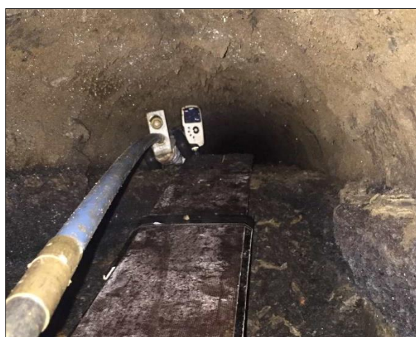
Photo 4 – A camera sitting on top of the trolley at the winding pit end of the drain - note the depth of silt. (© D Hore, 2022)
