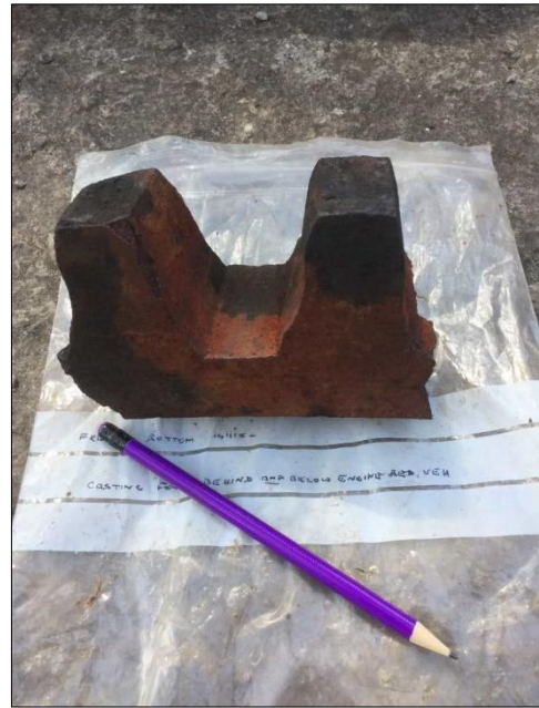
Photo 32 – ... and in 2022 after cleaning when it was found to be part of a gear wheel – see comments on p.3. (© H Orr-Ewing, 2022)
