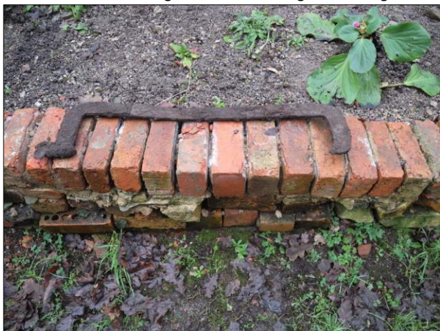
Photo 23 – The large hacksaw frame found in the New Boiler area. Made from a 2" wide metal strip, it is 30½" long overall.
