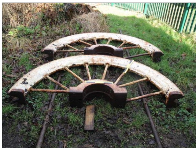
Photo 5 – The two halves of the 6' 6" diameter wheel that came from the Calverton Colliery via the SGMRG. (30 cm black/yellow scales on the near half)
