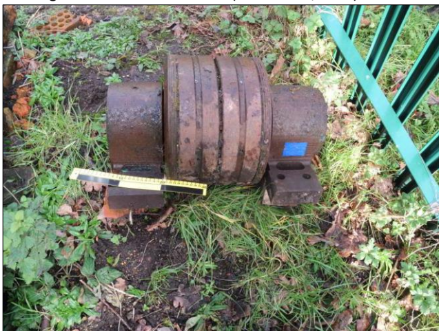
Photo 29 – Bearing for the 6' 6" diameter wheel. The blue patch on the right is the manufacturer's sticker, seen in close-up below. (30 cm black/yellow scale)
