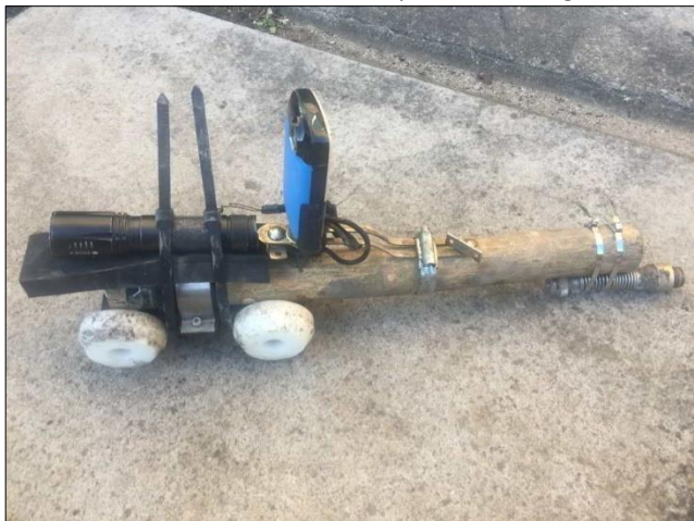
Photo 24 – Derek's remote survey trolley when rigged for photography. Light came from the torch strapped to the left hand end. (© D Hore, 2022)
