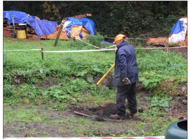
Photo 15 – Derek using a magnetometer to search for metal objects in the area where the refreshment tent stood during the HOD weekend ...
