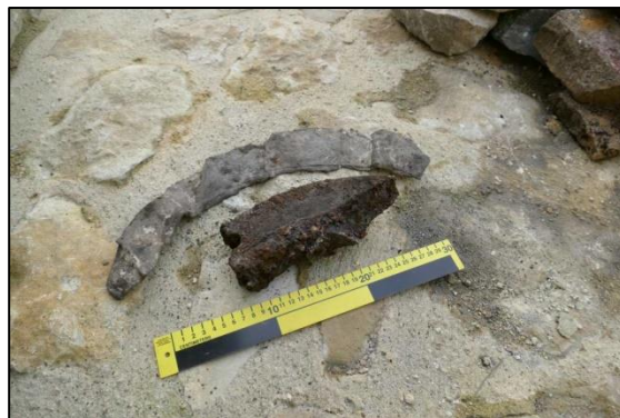
Photo 18 – These objects were also found in the excavated spoil. The bottom item appears to be part of a flange of a large diameter pipe (BB 130219-1), while the strip of lead above it may have been part of a gasket (BB 130219-2). (30 cm scale)
