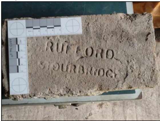
Photo 32 – Tapered firebrick, found in the under croft of the Horizontal Engine House, with the maker's mark 'Rufford Stourbridge' stamped onto one face. A similarly marked brick was found in the Vertical Engine House in 2016. The other tapered firebricks found, with the exception of the one seen below, have not been marked with a maker's name.
