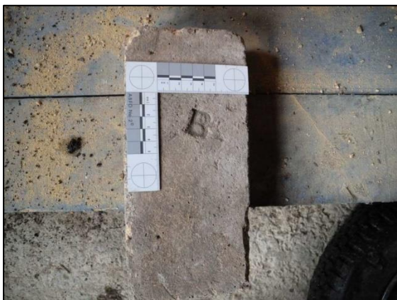
Photo 33 – Tapered arch firebrick, found in the under croft of the Horizontal Engine House, with the maker's mark 'B' stamped onto one face.
