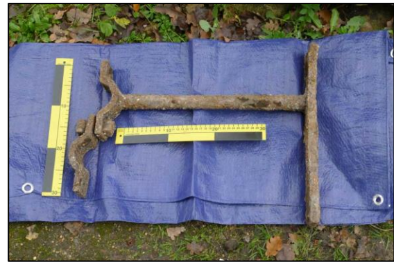
Photo 10 – Iron pipe support, found at the south-eastern end of the East Flue. The central rod is 16" long, and the clamp on the left could accommodate a 2" diameter pipe when fully closed. (30 cm scales)
