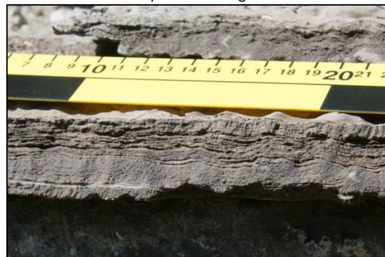
Photo 5 – Close-up of the edge of a sample of the scale seen in photo 4, which has been deposited over time in irregular layers.
