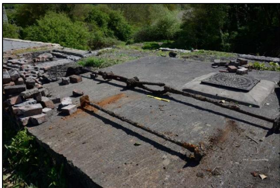
Photo 20 – The wire rope and anchorage point, seen in the middle of the photo, after removal from the trench. (30 cm scale below the loop in the wire)
