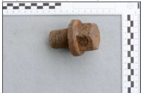
Photo 60 – 2½" long plug found in the flywheel slot, Vertical Engine House. (140516-3, 30 cm x 15 cm scale)
