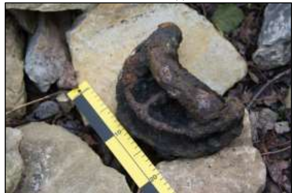
Photo 65 – Fragment of a spoked wheel, probably from a coal tub, found in the southern tippler slot of the Old Pit heapstead. Cleaning of-site separated the length of bent pipe (on top) from the remains of the wheel.
