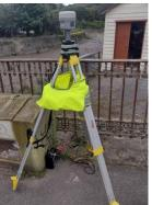
listening to up to 30 GPS satellites so as to accurately calculate its position in three dimensions.
