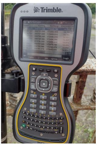
A roving staff with another GPS-sensing head recorded the location in space of each bollard, building, plate and dock coping as required. The roving GPS continually corrected its location by communicating with the base unit, so that it knew where it was to an accuracy of less than a centimeter. It reported its accuracy to Charlie continuously, (generally within 8mm) and refused to work if its error exceeded 30mm. (1 1/2ins).
