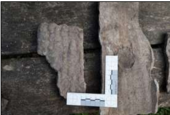
Photo 20 – Two more pieces of lime scale from elsewhere in the channel. The rough surface of the one on the left would have been in the flow of water, while the smooth surface of the one on the right was against the wooden edge of the channel. (5 cm x 5 cm scale)
