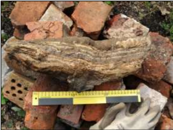
Photo 19 – Close-up of another piece of limescale found in the channel in the bob wall, with more layers of lime scale build up. (30 cm scale)
