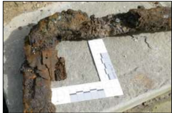
Photo 11 – Remains of what appears to be a leather gasket attached to part of the frame seen in the photo on page 2. (5 cm x 5 cm scale)
