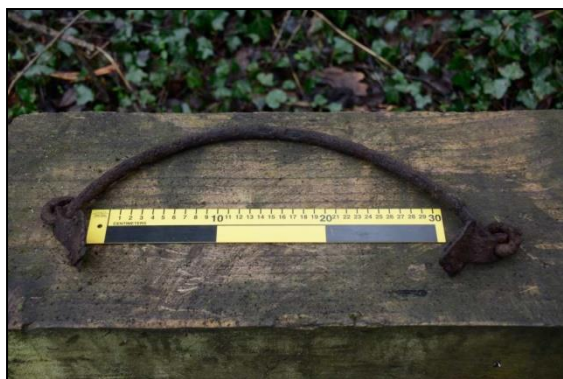
Photo 1 – 16¾" long metal handle found near the tippler slots, Old Pit heapstead. With a bowed height of 5½", it was secured by two triangular plates fitted to the swivels at each end. (30 cm scale)
