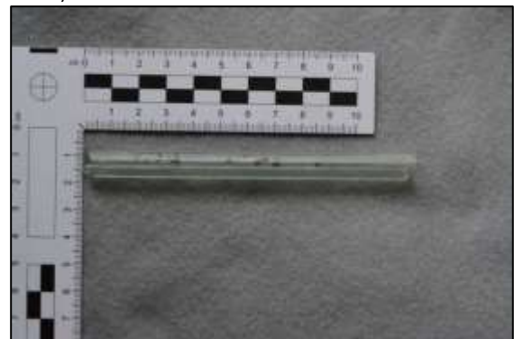
Photo 9 – 4¾" long piece of glass tubing that may have come from a manometer, found in the pit below the engine bed, Vertical Engine House. (10 cm x 10 cm scale)
