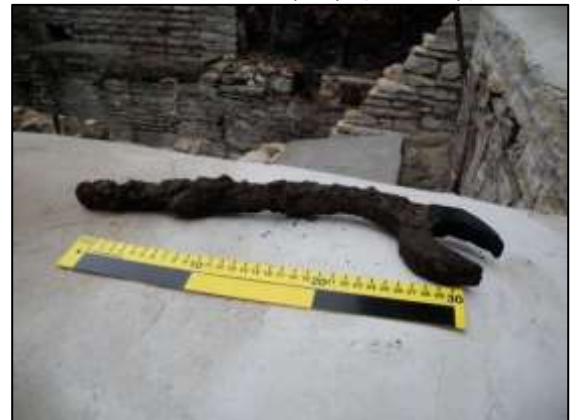
Photo 15 – 15” long spanner, with 1½” wide jaws, found in engine bay pit, Vertical Engine House. (30 cm scale)
