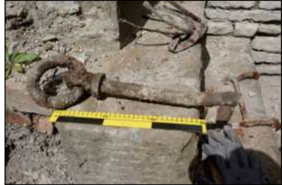
Photo 9 – 15" long eye bolt with a 5½" diameter ring at one end. The other end has been threaded. (30 cm scale)
