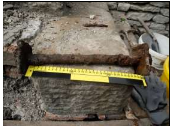
Photo 10 – 15¼" long bolt before cleaning. (30 cm scale)
