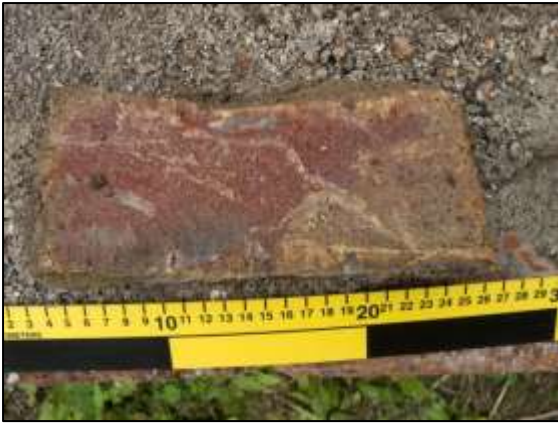
Photo 18 – The marbled appearance of the freshly broken face of a piece of buff-coloured building stone ...
